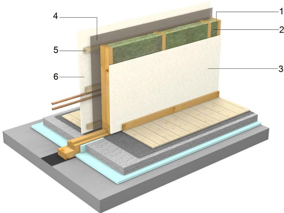
1- Structure bois: elements prefabrique, traitee CL2,a 15% d' humiditee, rabotee
